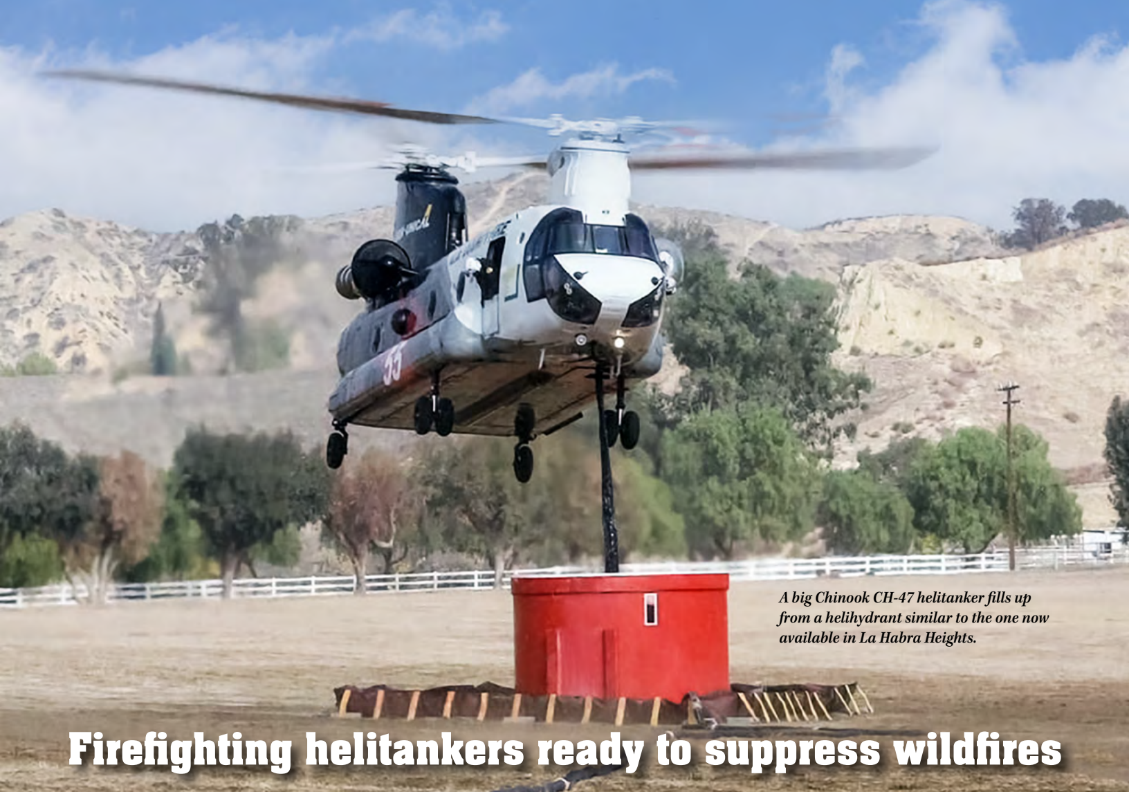
Each helitanker has a 3,000-gallon tank. (Coulson illustration)
