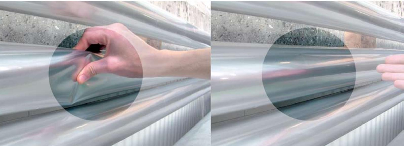
*Isogenotec® responds flexibly to mechanical stresses, automatically resumes its former shape and shows no signs of damage.*
