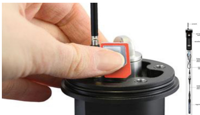
Figure 3—Wireless transmitter sim card installation (Morton, 2020)
