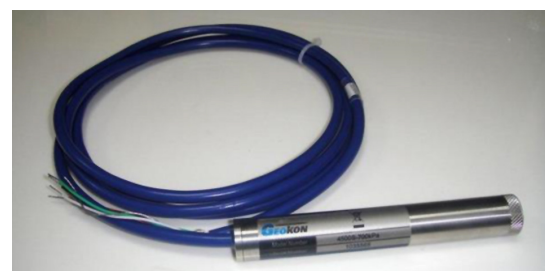
Figure 2—Example of a vibrating wire piezometer prior to insertion (Morton, 2020)
