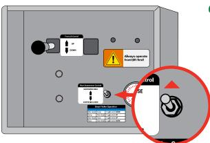
6. Push the rear suspension control smart-valve toggle switch to the "SUSPENSION RAISE" position for 1 second to raise the rear suspension.
