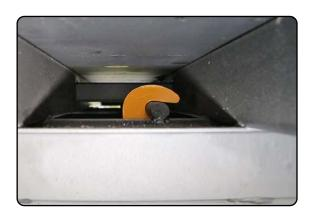
1. Each set of hooks must be undamaged, working correctly, and the container must be locked onto the chassis.
