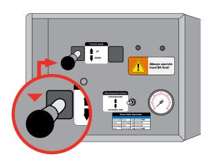
19. Return to the lifter control box and hold the front lift control lever in the "DOWN" position to lower the front lift assembly.
