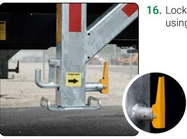
**16.** Lock the lower leg section in place using the yellow handle.
