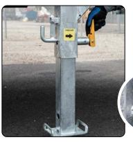
17. Lock the lower leg section in place using the yellow handle. The rear leg is now deployed.
