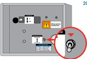
20. Push the rear suspension control smart-valve toggle switch down to the "SUSPENSION LOWER" position for 1 second to lower the rear suspension to ride height.
