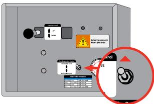
5. Push the rear suspension control smart-valve toggle switch up to the "SUSPENSION RAISE" position for 1 second to raise the rear suspension.
