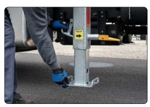
12. Release lower leg gravity lock and lower the lower leg section using the footpad handle.
