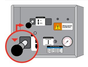
18. Return to the lifter control box and hold the front lift control lever in the "DOWN" position to lower the front lift assembly.
