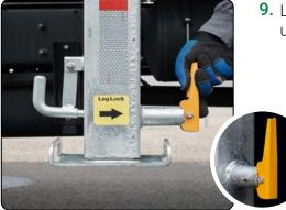
**9.** Lock the lower leg section in place using the yellow handle.
