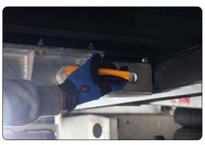
8. Unlock the top leg section using the yellow handle to disengage the spring lock pin.
