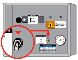
19. Push the suspension control smart-valve toggle switch down to "SUSPENSION LOWER" for 1 second to go from raised to ride height.
