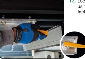
**12.** Lock the top leg section into place using the yellow handle. **This will lock the entire leg into place.**
