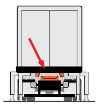
**3.** Be sure the chassis is aligned straight in front of the container.
