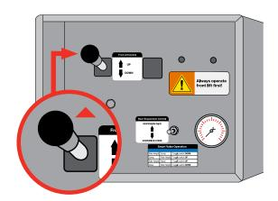
5. ALWAYS operate the front lift assembly first. At the lifter control box hold the front lift control lever in the "UP" position to raise the front lift assembly.
