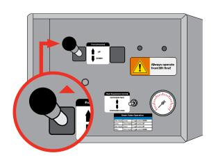
4. At the lifter control box hold the front lift control lever in the "UP" position to raise the front lift assembly.
