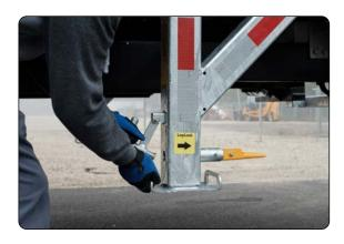
16. Release the lower leg gravity lock and lower the bottom leg section using the foot pad handle
