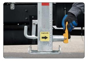
11. Unlock the lower leg section using the yellow handle to disengage the spring lock pin.
