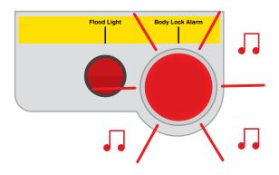
3. The in-cab alarm must work properly. When container is unlocked the alarm sounds and flashes.
