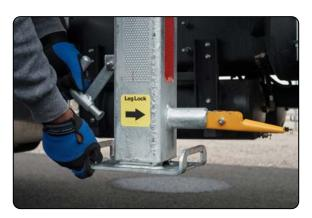
Release lower leg gravity lock and raise the lower leg section using the foot pad handle
