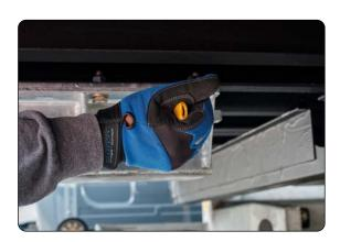
Unlock top leg section under container using the yellow handle to disengage the spring lock pin.
