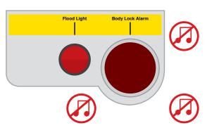
**22.** When the locking hooks are engaged the alarm on the dash will stop flashing and sounding.
