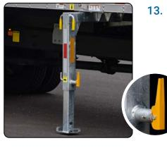
Lock the lower leg section in place using the yellow handle. The leg is now deployed.
