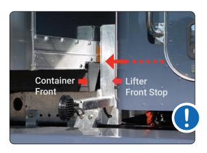
**4.** Slowly back the truck straight under the container until the front stops on the lifter contact the front of the container.
