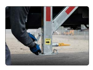
**15.** Release lower leg gravity lock and raise the lower leg section using the foot pad handle.
