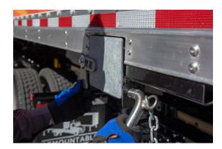
All legs must be properly stowed with leg pins secured. The secondary locking mechanisms must be in place.
