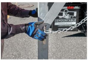
Insert the leg pin through the brace and leg. Swivel the handle down to secure it.
