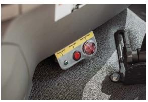
18. When the locking hooks are engaged the alarm on the dash will stop flashing and sounding.
