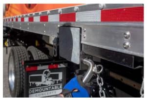
15. Rotate the handle portion of the leg pin upward and slide it out of the leg and retainer.
