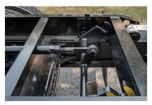
Make sure the locking hooks are in the unlocked and down position.
