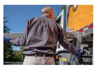
Lift the vertical portion of the leg to a horizontal position and slide the entire leg into the leg housing.
