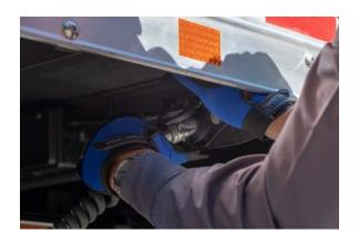
The light plug must be plugged into the container and lights must be functional.
