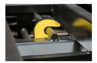
Each set of hooks must be undamaged, working correctly, and the container must be locked onto the chassis.
