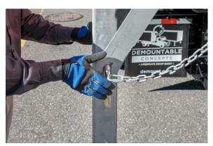
17. Insert the leg pin through the brace and leg. Swivel the handle down to secure it.
