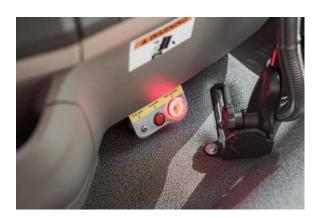
The in-cab alarm must work properly. When container is unlocked the alarm sounds and flashes.
