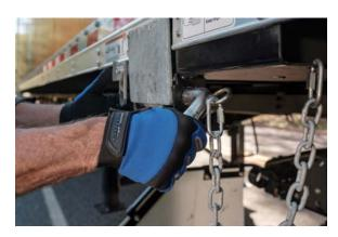
Rotate the handle portion of the leg pin upward and slide it out of the leg and retainer.
