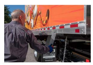
11. Lift the vertical portion of the leg to a horizontal position and slide the entire leg into the leg housing.
