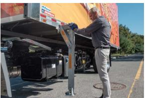
11. Push the leg assembly into the housing until the top brace touches the container side rail.
