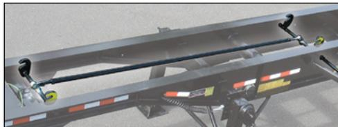
◀ Body lock-down mechanism on Semi-Trailer.
