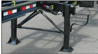
Heavy-duty crank-down landing gear with shoes.
