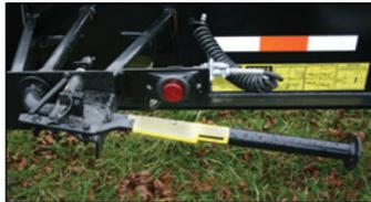
Body lock down lever with lockable safety key and improper lock-down warning light.
