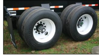
5/8" wall, 5" round tandem axles with hub odometer. Rated to carry 22,000 lbs per axle.
