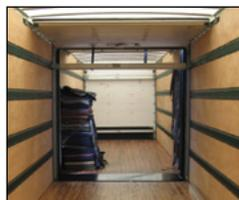
Walk-through front and rear doors allow multiple bodies to be loaded at the same time
