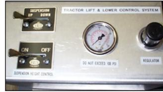
Air suspension lift and lower controls are mounted inside the tractor's cab.
