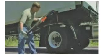
Lower center stops and unlock rear body utilizing locking lever. Slide legs out of the bodies. Adjust to compensate for uneven locations and lock into place. Repeat process for each body.
