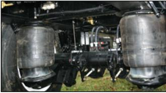
Tandem air suspension - lifting lowering capability of 25,000 lbs per axle.
