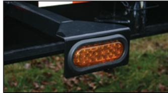
LED turn signal mounted at middle of both sides of trailer.
