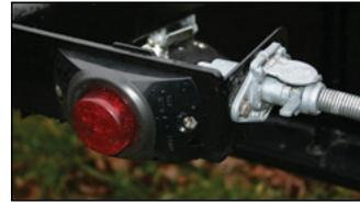
Electrical connection between body & trailer and improper lock-down warning light.
