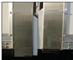
3" spacing between bodies. Poly-bumpers on front and rear of body.
