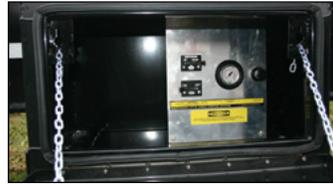
Lift and lower controls mounted inside a steel box on trailer's driver side.
