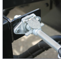
4- or 7-way connector to power interior and exterior lights on body.
