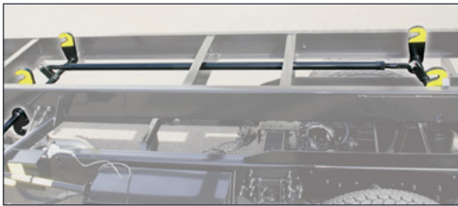
Four top and four bottom steel over-center body locking hooks secure body to the Chassis Lift Frame and Lift Frame to Truck Chassis.
