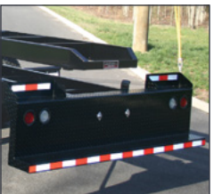
Heavy-duty, full-coverage rear step bumper with LED lights and white and red reflective tape.
