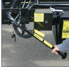
Body lock-down lever for securing and releasing body locking hooks.
