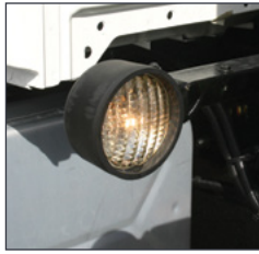
Rear-facing flood lights wired to dash or toggle switch.
