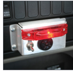
Dash mounted safety cut-off switch and lock warning light/buzzer.
