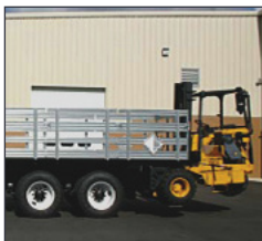
Piggy back option for transporting forklift with truck. Also shown: rear tandem axle/wheel option for heavy payloads.
