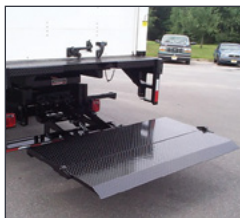
Tuck-under hydraulic lift gate mounted to truck chassis in lieu of a bumper. Utilize with all demountable truck bodies.
