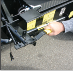
Lock lever and pad-lockable safety key keep body lock-down lever in correct position.
