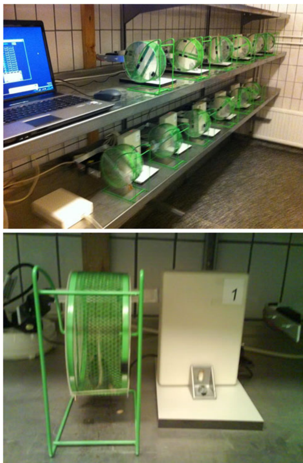
Fig. 1 Rodent running wheels with computer-controlled devices adapted for measurement of running exercise per unit time (Ödman et al. 2013) by individual mice over 30-min daily exercise sessions (Mondays, Tuesdays and Thursdays) or 10-min (Friday) or 30-min (Wednesday) test sessions. The arm of the upright (1) registers every revolution which is fed into a laptop computer that monitors all running activity by each mouse during the wheel-running session
