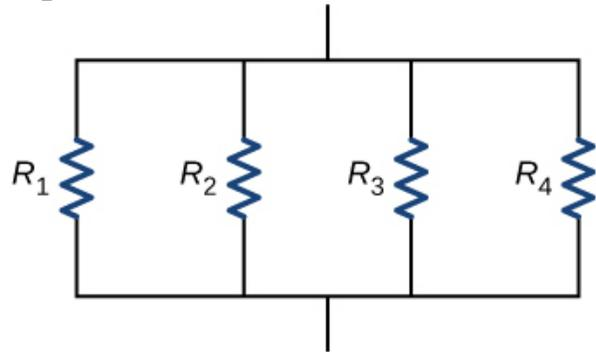
(b) Resistors connected in parallel
