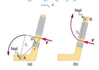
The third condition necessary to achieve equilibrium is that the net external torque on a system must be zero
