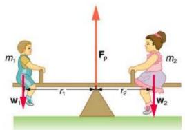
A system is said to be in **stable equilibrium** if, when displaced from equilibrium, it experiences a net force or torque in a direction opposite to the direction of the displacement
