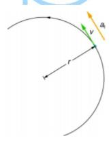
The **kinematics of rotational motion** describe the relationships among rotation angle, angular velocity, angular acceleration, and time
