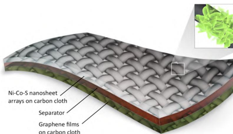
**Figure 1.** Schematic of the design of asymmetric supercapacitors by applying interconnected Ni–Co–S nanosheet arrays on carbon cloth as a positive electrode and porous graphene film as a negative electrode.
