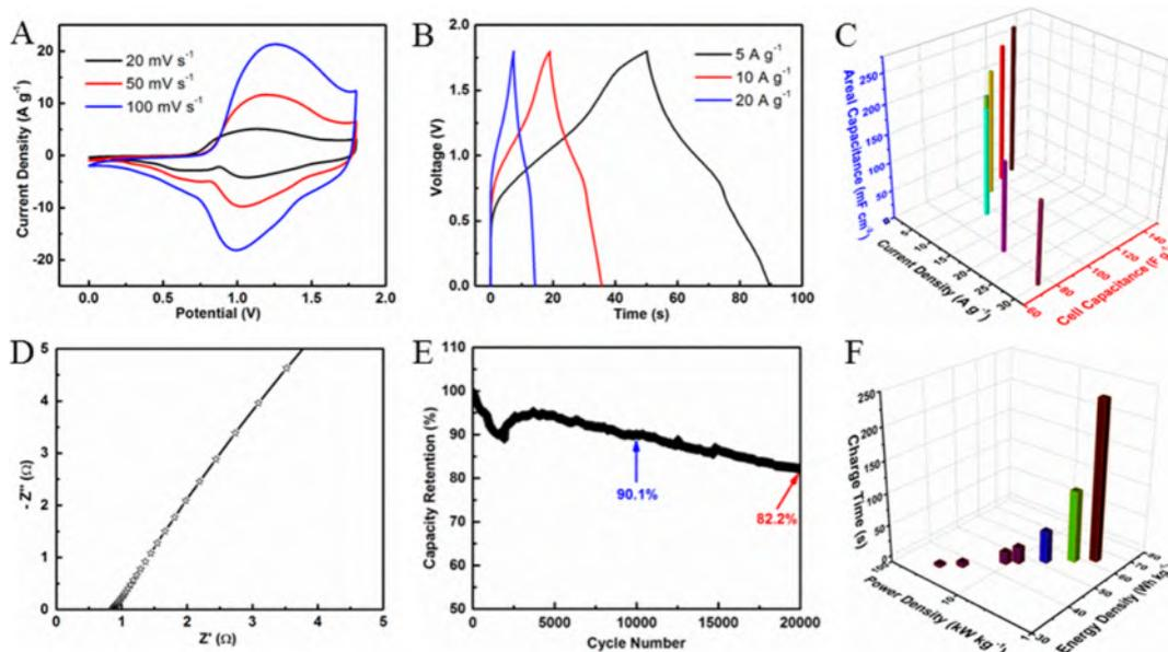
Figure 5. Electrochemical performance of the Ni–Co–S/graphene asymmetric supercapacitors. (A) Cyclic voltammetry curves; (B) galvanostatic charge–discharge curves; (C) cell capacitance and areal capacitance vs current density; (D) Nyquist plot; (E) cycling stability performance; (F) Ragone plot (energy density vs power density vs charge time).
