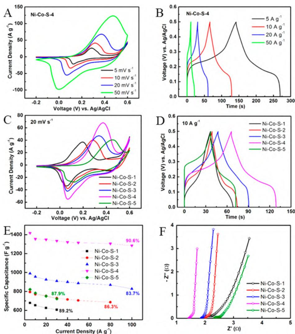
**Figure 4.** Electrochemical performance of the Ni–Co–S nanosheets as supercapacitor electrodes in the three-electrode measurements with 1 M KOH as the electrolyte. (A) Cyclic voltammetry and (B) galvanostatic charge–discharge curves of the optimized Ni–Co–S-4 nanosheets; (C) cyclic voltammetry, (D) galvanostatic charge–discharge curves, (E) summary of specific capacitance as a function of current density, and (F) Nyquist plot of all the Ni–Co–S electrodes, respectively.
