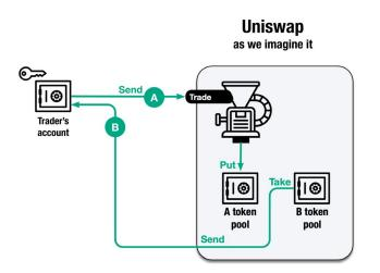
Conceptually, it is quite simple. Tokens are sent in, and the smart contract logic need only determine an amount of tokens to send back from its internal pool. Instead, here is a *greatly simplified* view of how just this one simple smart contract call works on the real Uniswap smart contract on Ethereum:
