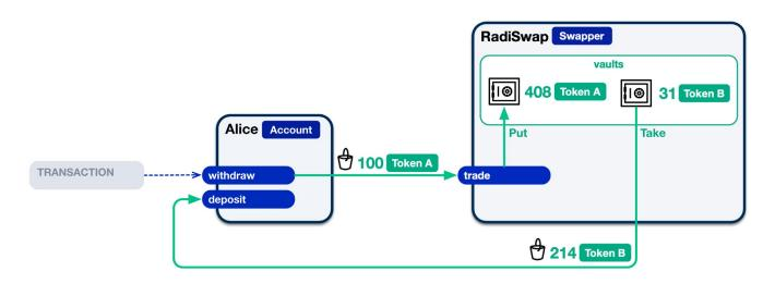
**Just as we imagined it to be!** Using Scrypto, the only code that needs to be written is an implementation of the *trade* method that looks at the incoming bucket of Token A resources, calculates the current exchange rate (based *directly* on the contents of its own internally-held pool vaults), and returns the right amount of Token B. All of the token manipulation performed by the *trade* method implementation happens via simple take/put functions on buckets and vaults.
