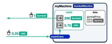
A bucket of 0.25 USD is passed to the *insertCoins* method of the *myMachine* component (previously instantiated from a *GumballMachine* blueprint), and the machine's logic sees that the correct price has been paid, puts those tokens in its USD vault, takes 1 Gumball from its Gumball vault, and passes it back to the caller. The component's logic might also send back change if the user passed in too much USD.
