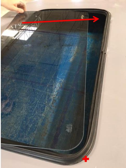
Start glass installation by sliding in a corner into gasket (+) and pivoting other side into opposing corner.
