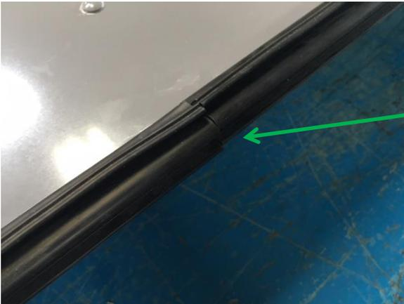
Make sure that the two ends meet up and touch flush.
