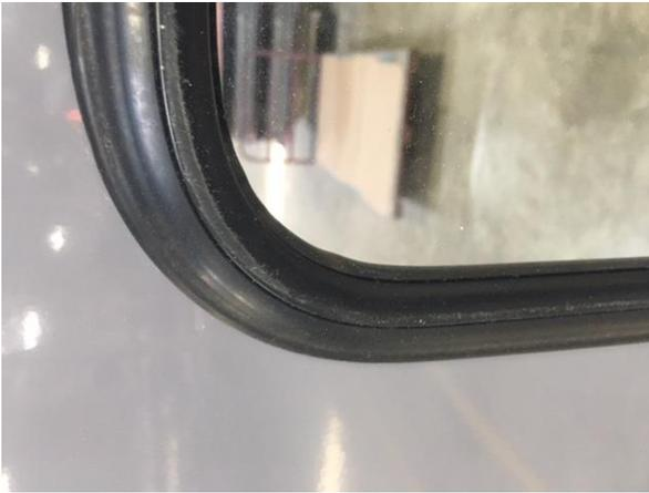
Inspect the corners to make sure that no wrinkles are visible and that the locking flap is tight.
