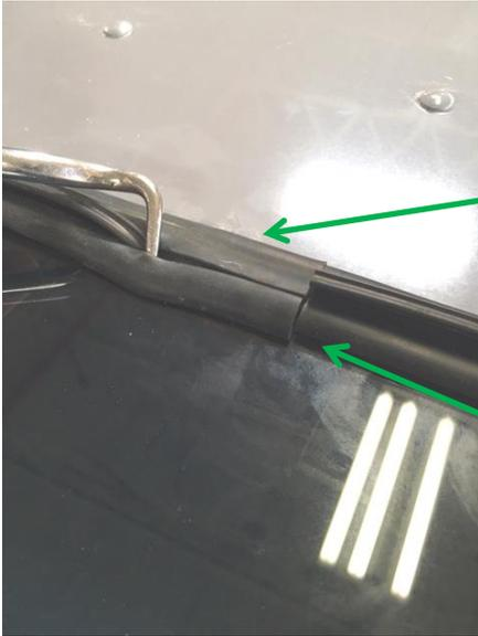
Once you get glass fully inserted into gasket, you will need to use the gasket tool to push the locking flap into the gasket around the whole window. This locks the window into place.
