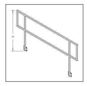
Material Steel ASTM A500
