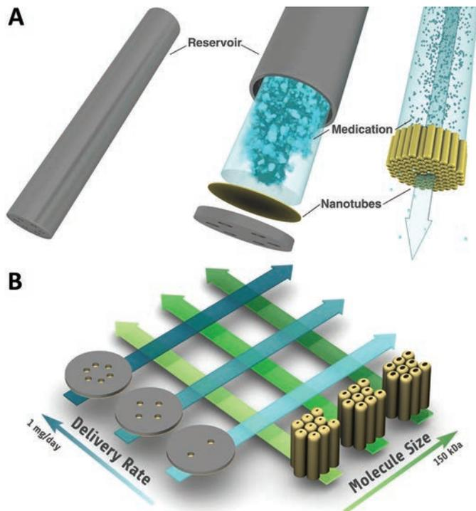
**Figure 2.** Schematic of NanoPortal implant. (A) Overview of device assembly. (B) Constant-rate delivery for a variety of molecules can be achieved by adjusting the size of the nanopores; target delivery rates can be achieved by adjusting the number of accessible nanotubes.
