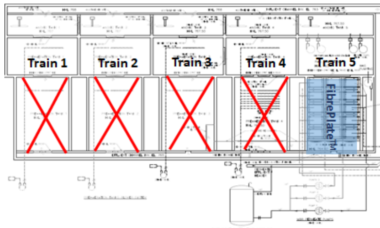
Figure 1.0 – Delphos train elimination with FibrePlate installation
