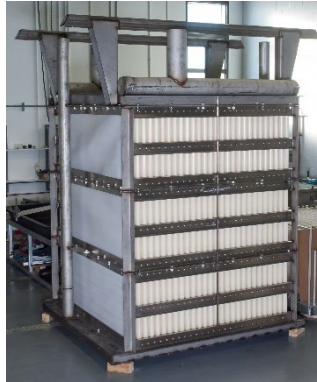
Figure 2.0 – FibrePlate 28-Module Cassette (42,000 ft 2 membrane area)
