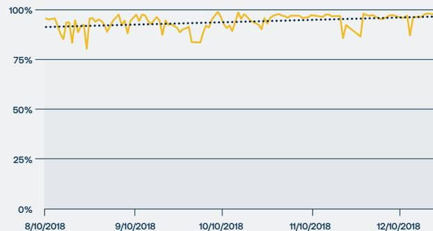
**Figure 2.** First-Step Anaerobic EcoVolt Reactor BOD Removal Efficiency (Before Second-Step Aerobic BlueCycle MBR Polishing)
