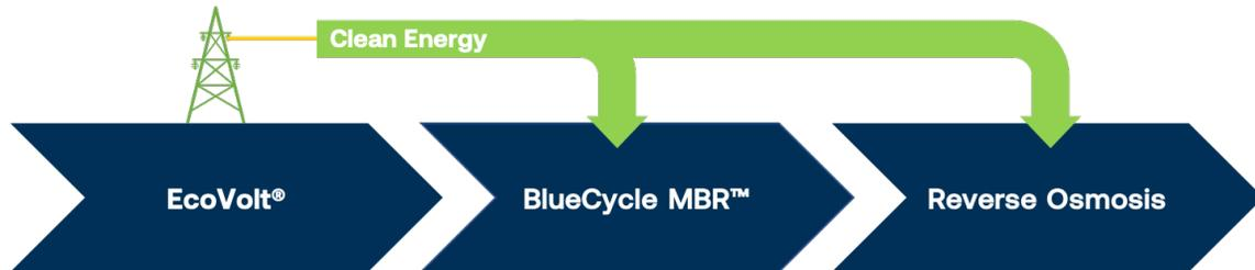
*Fig 2. Cambrian Self-Powered Wastewater Treatment Train*
