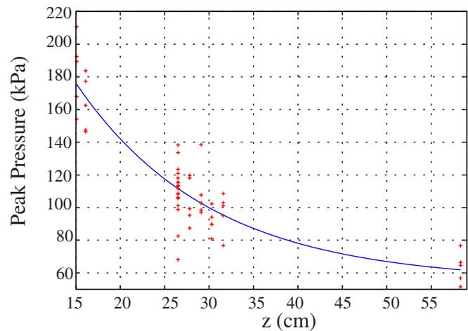
FIG. 3. (Color online) Characteristic height  $P_{\text{nom}}$  of pressure wave as a function of distance from the muzzle. Each point shows the pressure for a single shot. The curve is the optimum exponential fit,  $(330 \text{ kPa})e^{-z/(15 \text{ cm})} + 55 \text{ kPa}$ .
