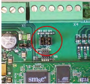
Figure 2 - RS-485 Termination Jumpers ON
