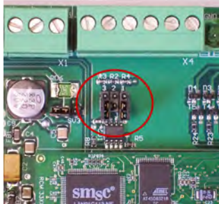
Figure 3 - RS-485 Termination Jumpers OFF
