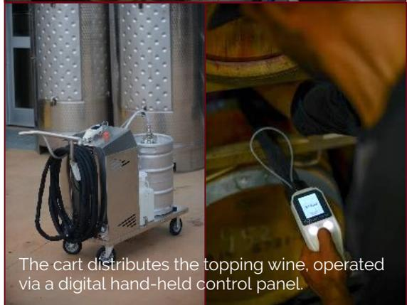
The cart distributes the topping wine, operated via a digital hand-held control panel.
