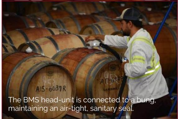
The BMS head-unit is connected to a bung, maintaining an air-tight, sanitary seal.
