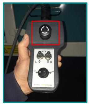
**NOTE:** Emergency stop on track controller will shutdown the engine and sound an alarm, but only if it is plugged in. Ensure E-stop is disengaged to activate the track controller.
