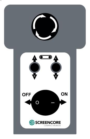
Move the machine's tracks via the up/down toggle switches. Independent operation of each track can be achieved with the forward and reverse positions.
