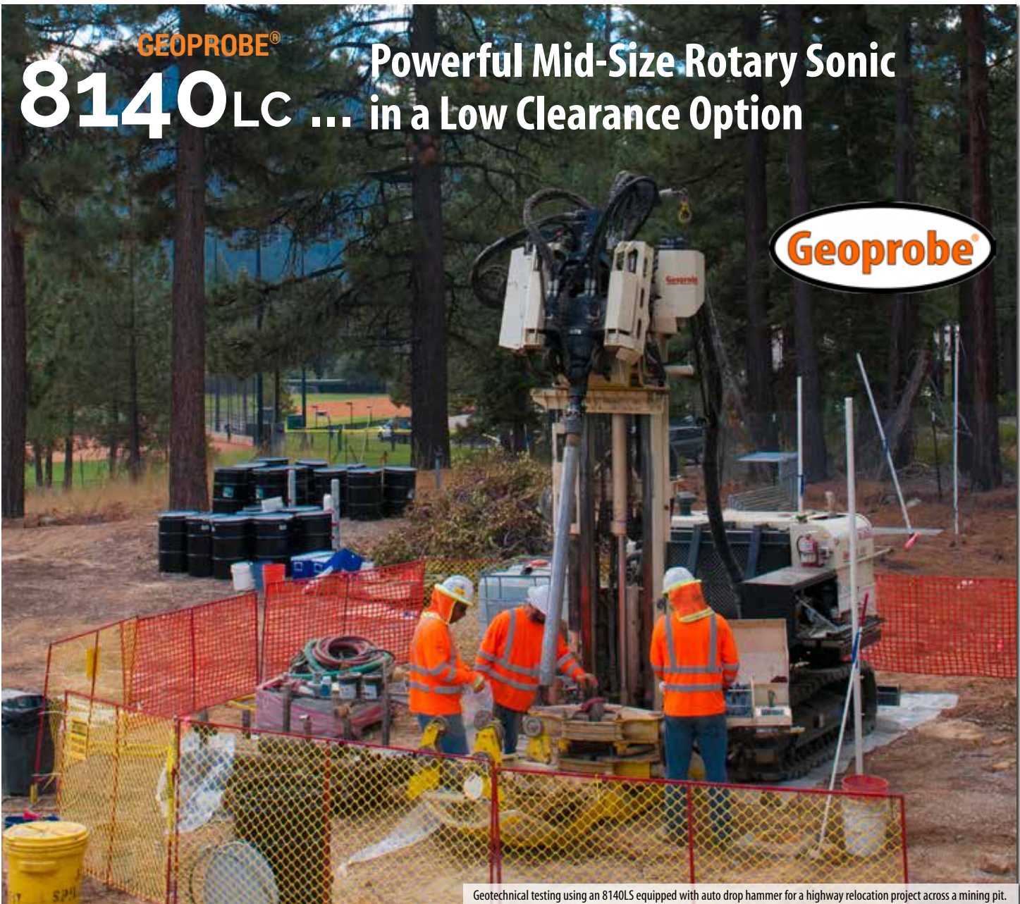
Geotechnical testing using an 8140LS equipped with auto drop hammer for a highway relocation project across a mining pit.
