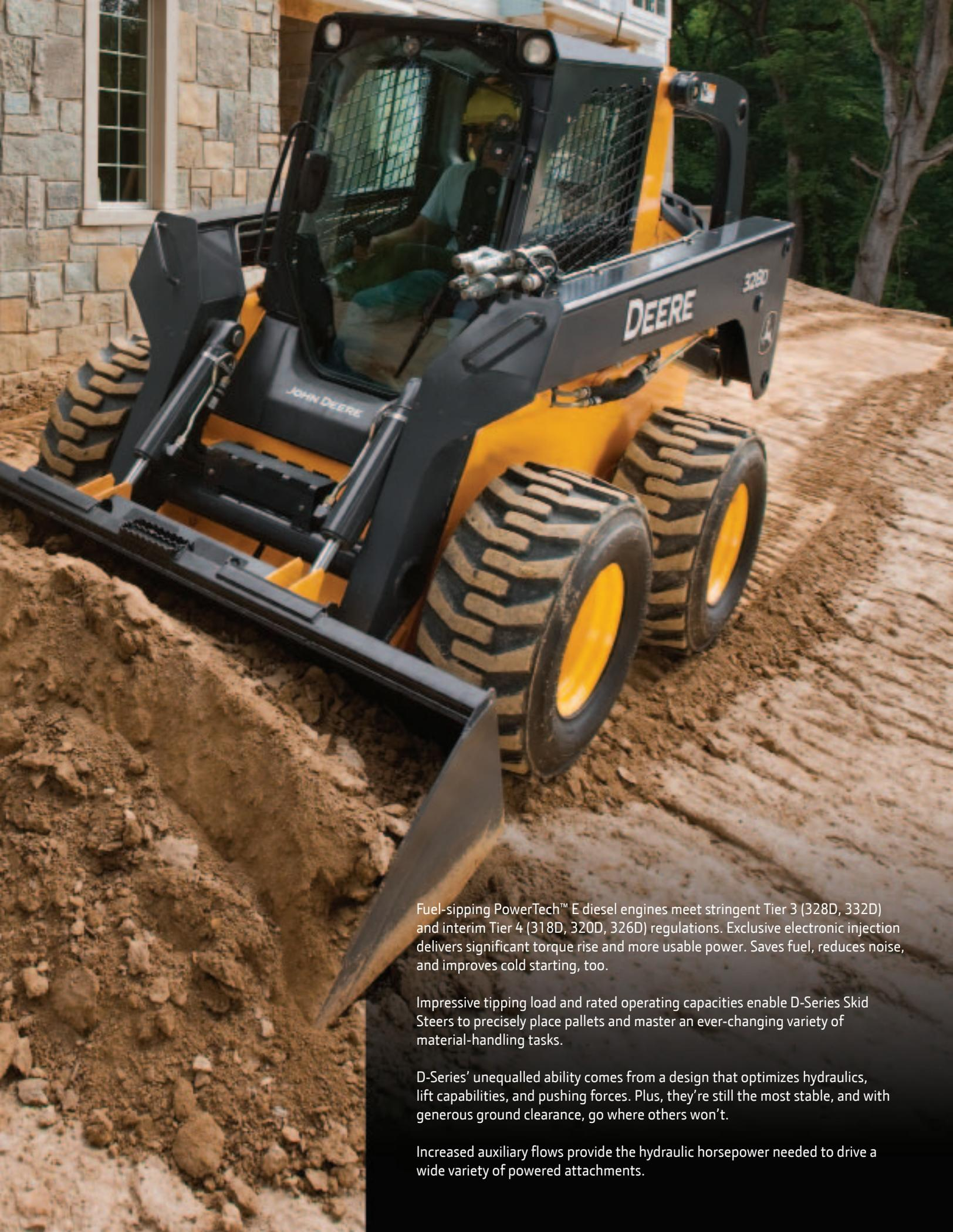
Fuel-sipping PowerTech™ E diesel engines meet stringent Tier 3 (328D, 332D) and interim Tier 4 (318D, 320D, 326D) regulations. Exclusive electronic injection delivers significant torque rise and more usable power. Saves fuel, reduces noise, and improves cold starting, too.
