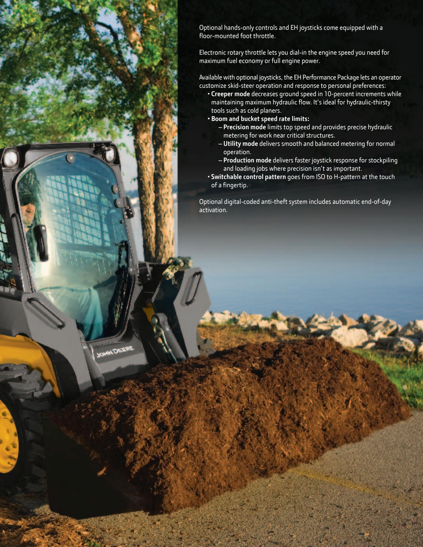
Optional hands-only controls and EH joysticks come equipped with a floor-mounted foot throttle.
