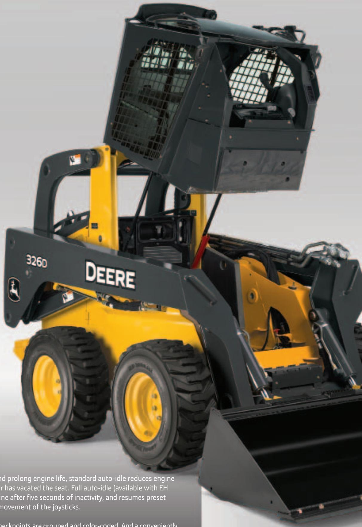
To help conserve fuel and prolong engine life, standard auto-idle reduces engine speed after the operator has vacated the seat. Full auto-idle (available with EH controls) slows the engine after five seconds of inactivity, and resumes preset engine speed with any movement of the joysticks.
