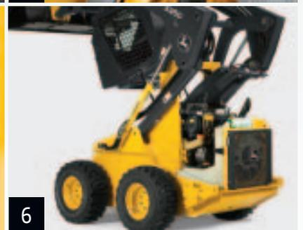
1. Daily servicing is quick and convenient. Simply lift the hood for ground-level access to check fluids and refuel.
