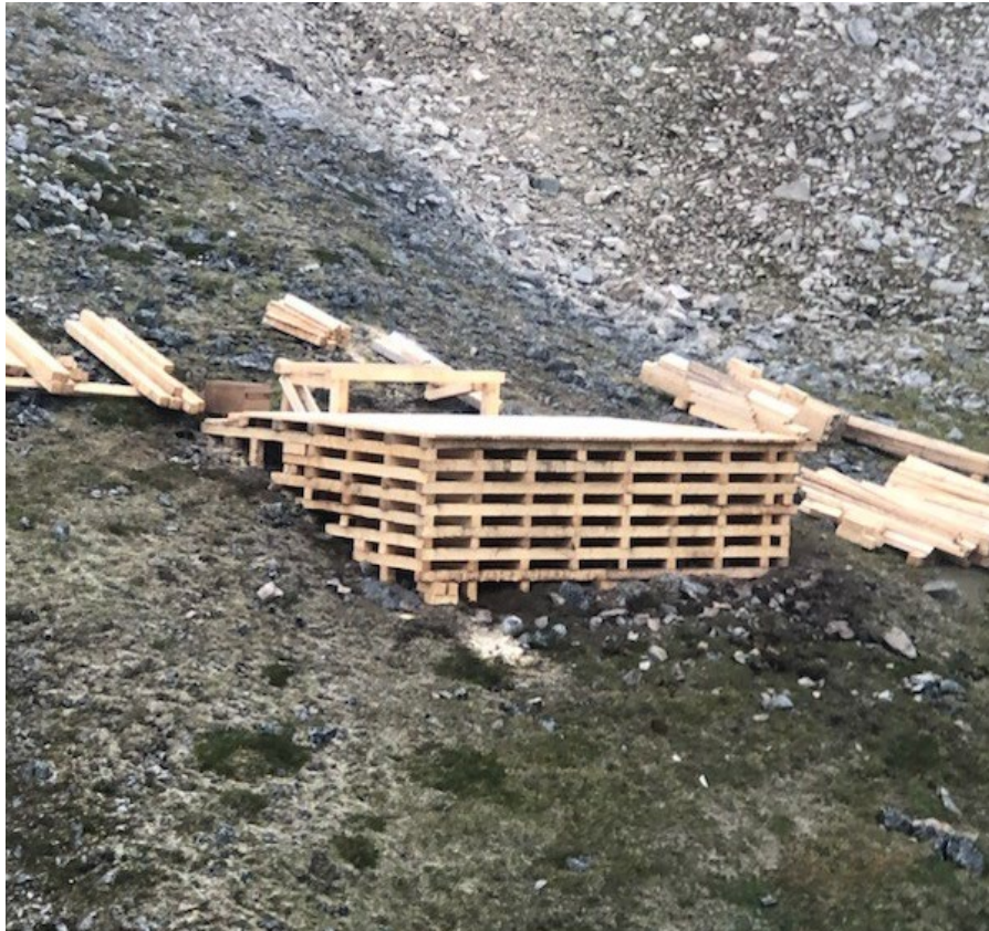
Figure 2: Pad used to drill a series of 12-15 drill holes on the Coleman Segment of the Lucky Shot vein.
