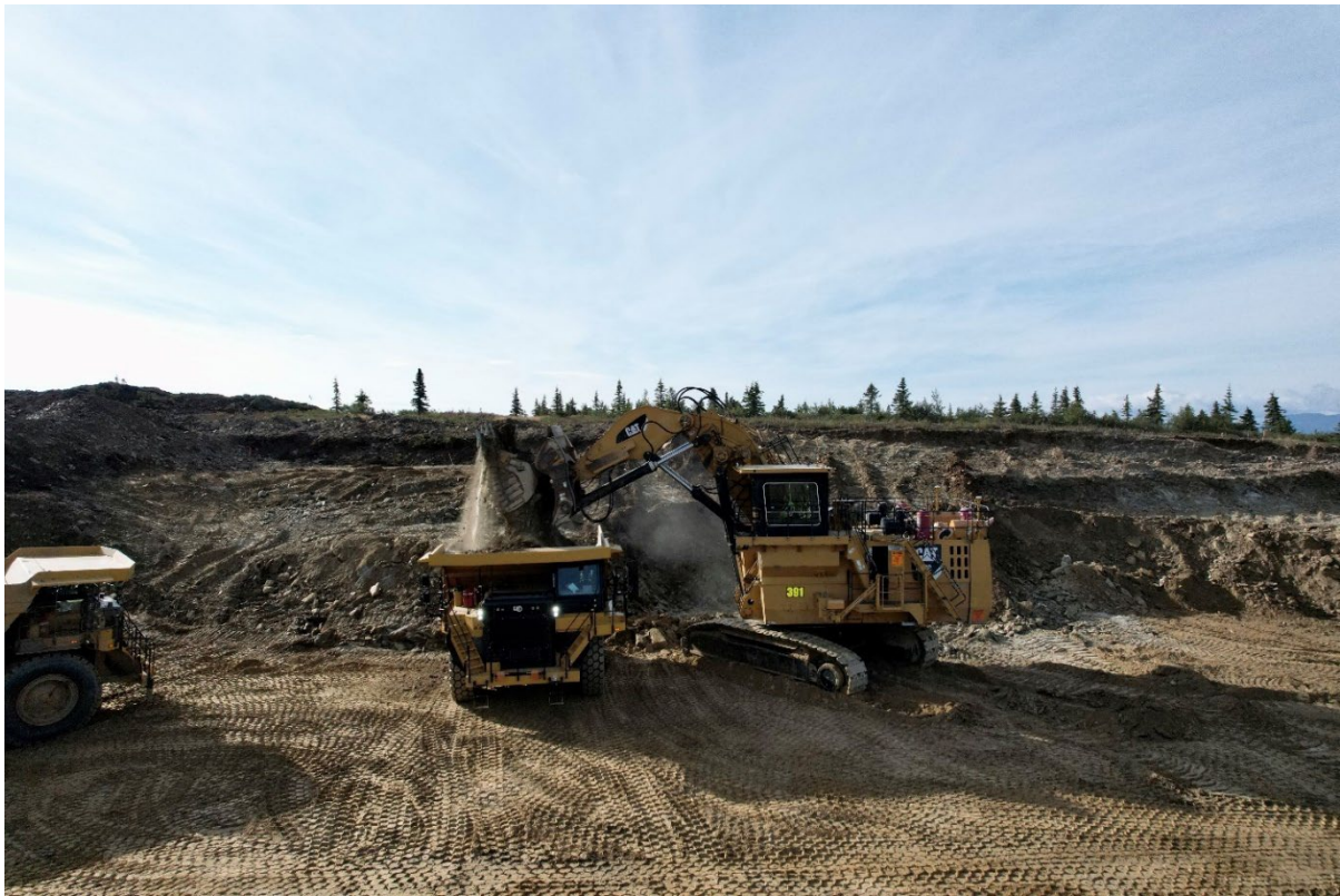
Figure 1: Photo of the CAT 6030 shovel loading a 777 CAT (85 ton) haul truck at Manh Choh Mine.
