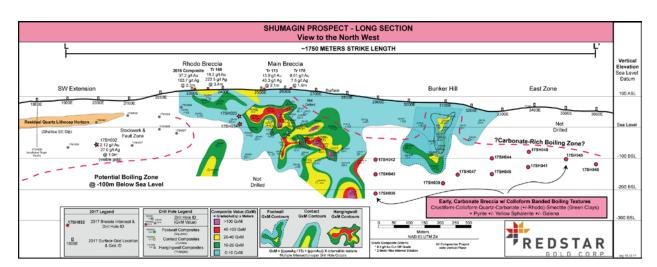
Figure 1: Long Section - Shumagin Gold Zone: Main Breccia, Bunker Hill and East Zones
