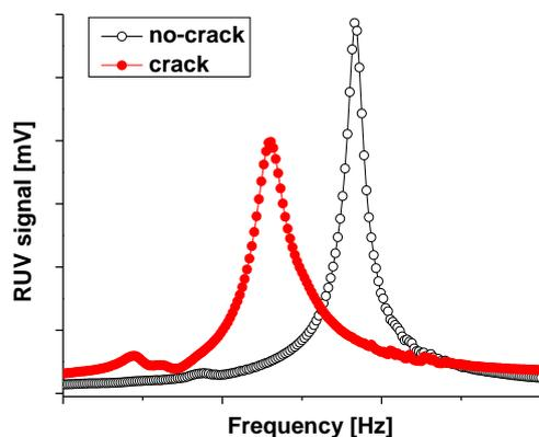
Figure 1: Deviations of RUV parameters caused by a crack
