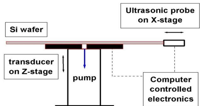
Figure 2: RUV schematic
