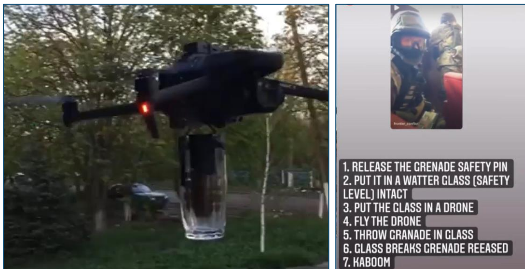
Figure 24: Instructions and use of DJI Mavic 3 drone to drop a glass with a grenade inside
