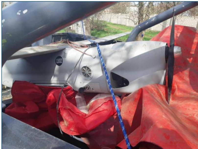
Figure 32: Orlan-10 drone (Tail Number: 12652) taken down via electronic warfare
