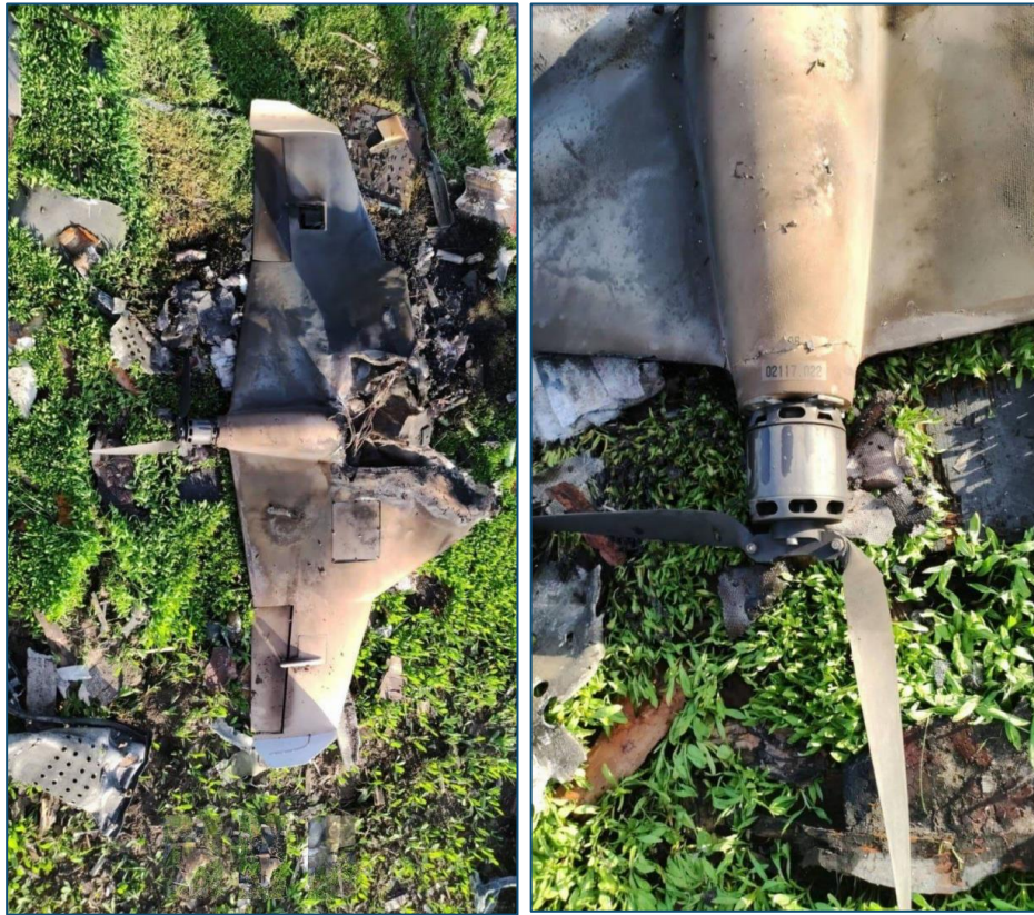
Figure 17: Russian suicide drone KUB-BLA with the tail number of 02117022
