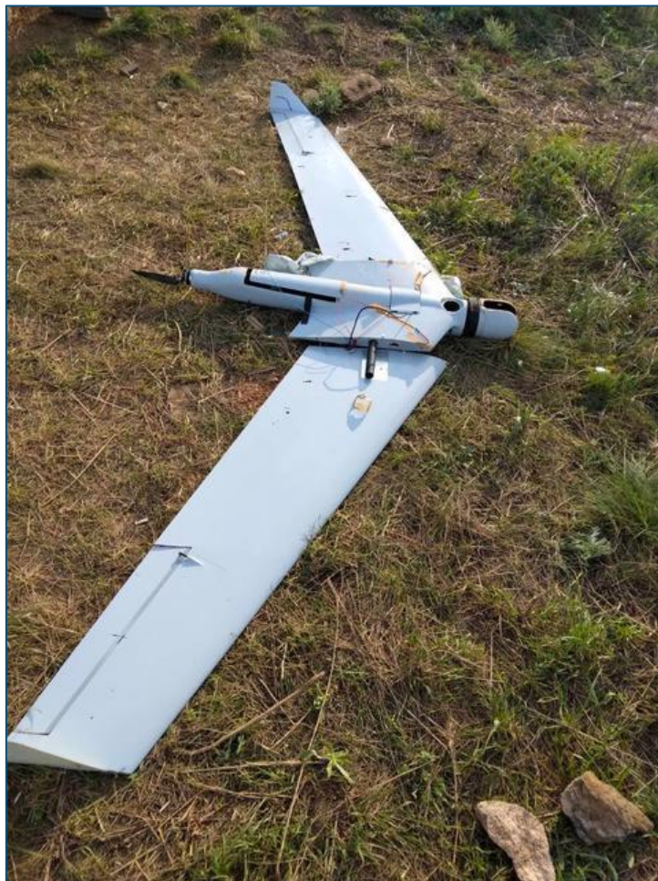
Figure 26: Russian Zala 421-16E drone shot down and seized
