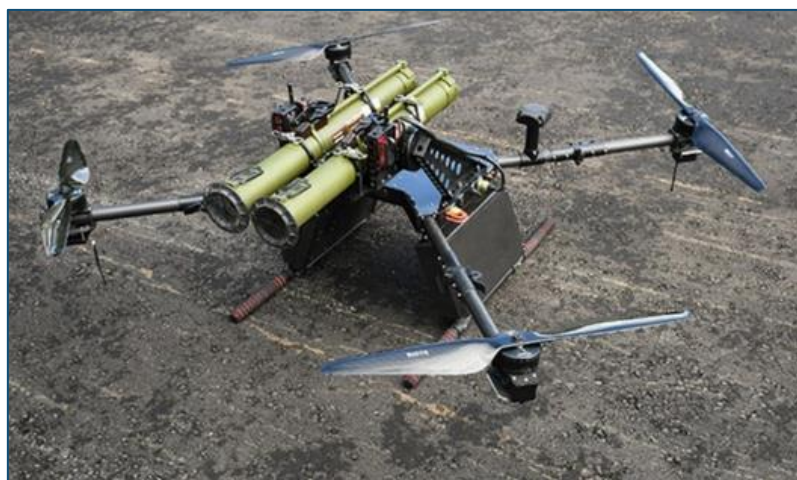
Figure 17: Kvarado-1400 drone with two RPG-26 rocket launchers
