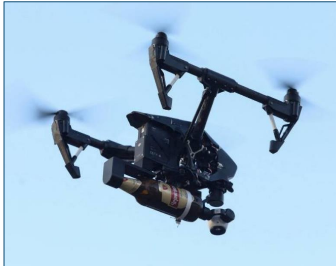
Figure 7: DJI Inspire drone modified to carry and release beer bottles sized incendiary munitions
