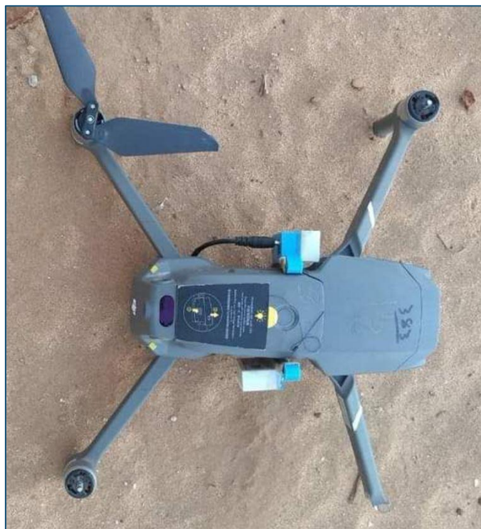
Figure 9: Houthi-owned DJI Mavic 2 drone with air dropping mechanism attached seized
