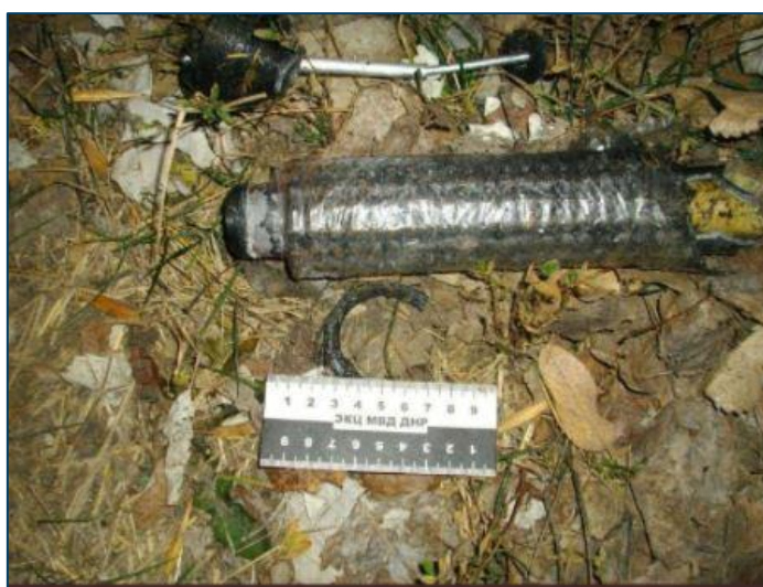
Figure 16: Explosives when detached from the R-18 drone
