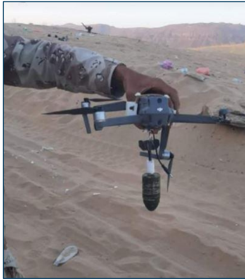
Figure 17: DJI Mavic drone with explosive warhead shot down by Yemeni forces
