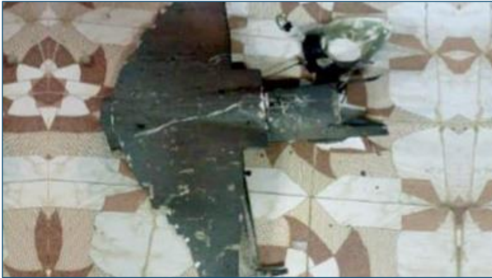
Figure 13: Remnants of destroyed Houthi delta wing drone over Jazan, possibly Qasef-1 drone
