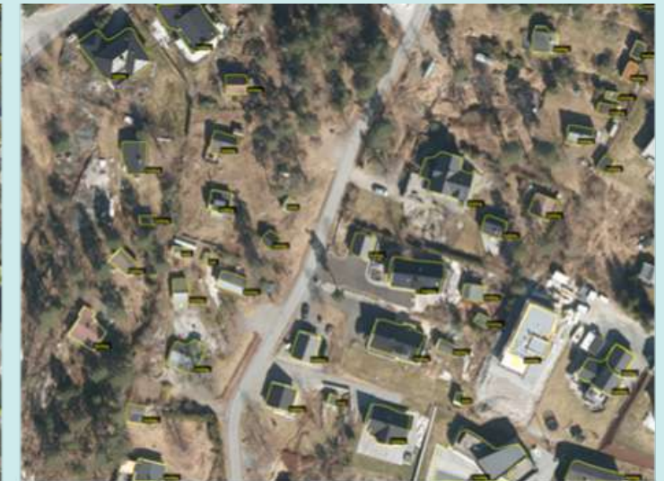
Photos: Aerial images and outlines (in yellow) of buildings in the Follo region. Left: Aerial image from 2018 and outlines used as 'ground truth'. Right: Aerial image of 2020 with automatically detected buildings. Notice the new building on the righthand side (with a bright ground surface around). (Terratec/NR).
