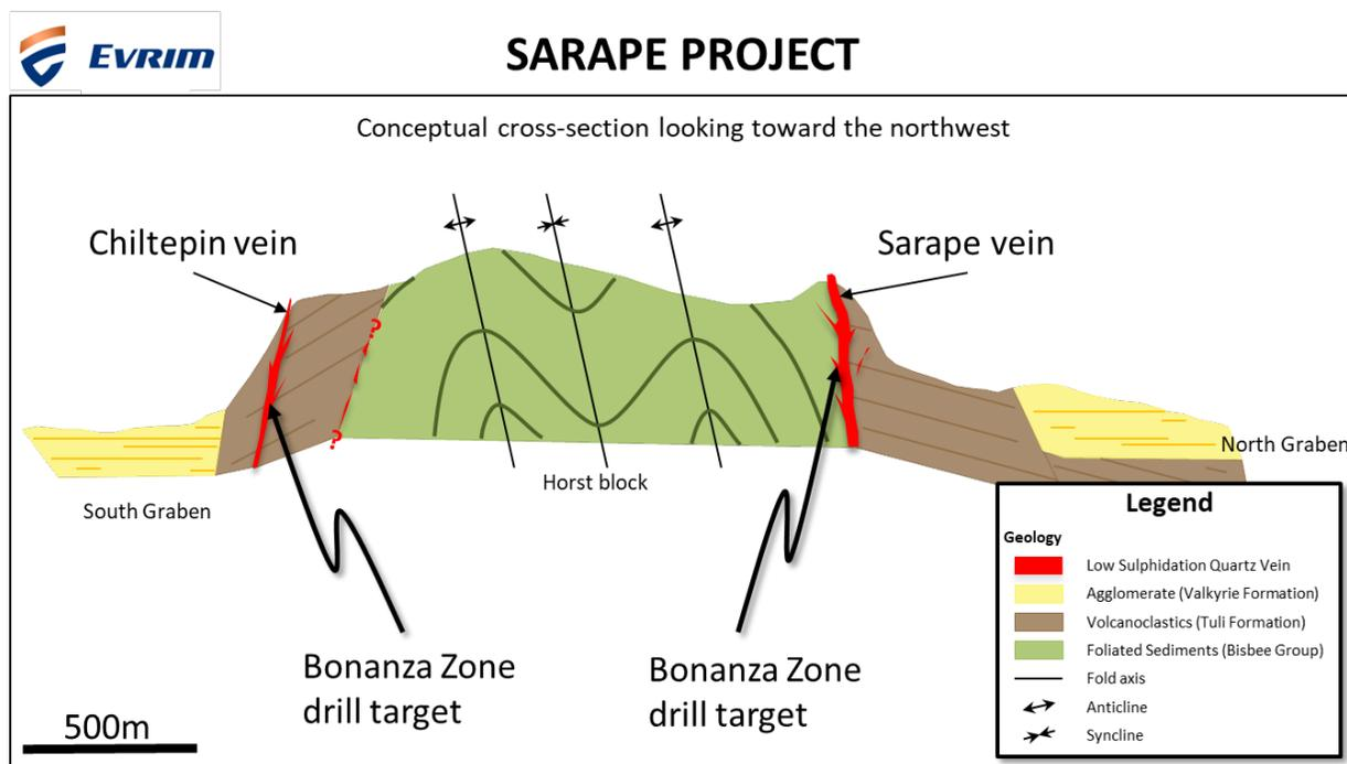
Figure 3 Conceptual cross-section
