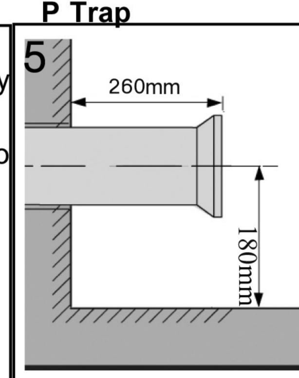
5.Set up waste pipe so that the end of the pan collar extends 260mm from the finished wall.
