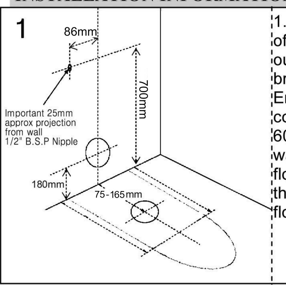
1.Rough in position of water inlet, waste outlet and floor fixing bracket holes. Ensure inlet connection extends 60mm from finished wall. Drill holes for floor fixing bracket then fix brackets to floor.
