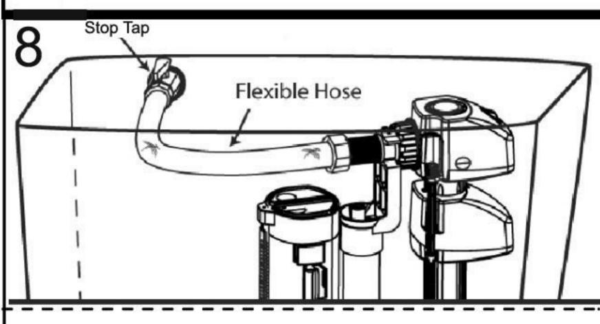
8. Fit off stop tap then connect rear water inlet valve to stop tap. Fill cistern and ensure correct water level.
