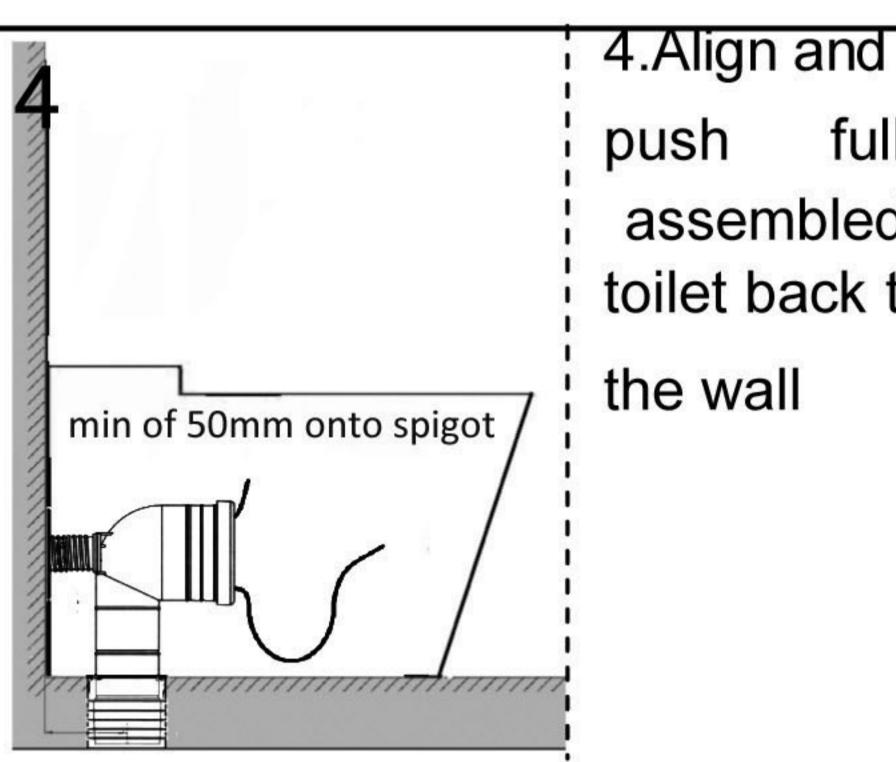
4.Align and push fully assembled toilet back to the wall
