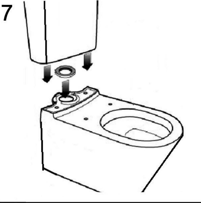
7.Place rubber seal into pan recess
