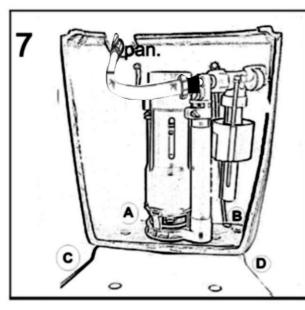
7.IF BACK INLET, SKIP THIS STEP. Remove cap from cistern plug A or B at base cistern. Connect flexible hose to cistern plug A or B depending on location of stop tap. Complete stop tap connection to underside of cistern plug C or D. Fill cistern and ensure correct water level.
