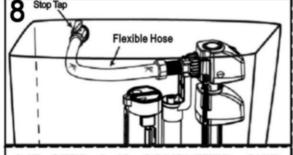
8.IF STEP 8 IS COMPLETED, SKIP THIS STEP. Fit off stop tap then connect rear water inlet valve to stop tap. Fill cistern and ensure correct water level.
