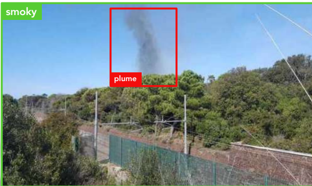
Proper smoky image classification with smoke plume detection (above) versus proper foggy image classification (below)
