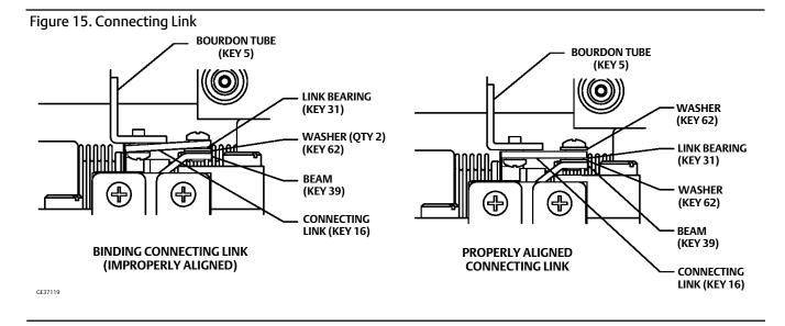
11. Check all tubing connections for leaks and the Bourdon tube machine screws, tighten as necessary. Perform the appropriate calibration procedures.
