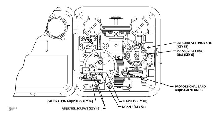
Connect a pressure source to the supply pressure regulator and be sure the regulator is delivering the correct supply pressure to the controller. The controller must be connected open loop (Open loop: The controller output pressure changes must be dead ended into a pressure gauge). The following procedures use a 0.2 to 1.0 bar (3 to 15 psig) output pressure range as an example. For a 0.4 to 2.0 bar (6 to 30 psig) output range, adjust the values as appropriate.
