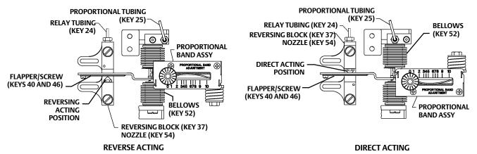
TO CHANGE ACTION OF THE CONTROLLER, REPOSITION THE PROPORTIONAL TUBING, REVERSING BLOCK/NOZZLE AND PROPORTIONAL BAND ASSY AS SHOWN ABOVE
