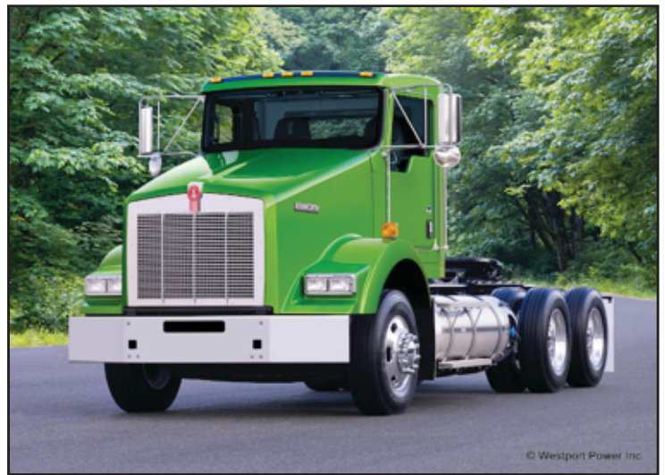
Kenworth T800 LNG factory-direct natural gas truck powered by Westport HD
