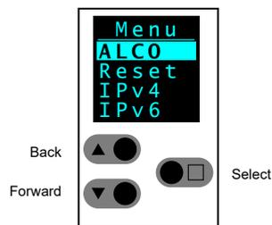
**Figure 42.** In-Shelf Controller Buttons: Horizontal Mount
