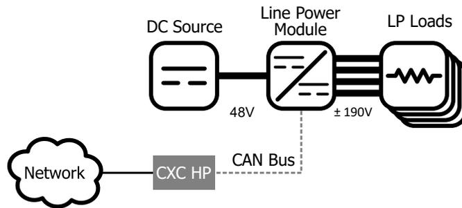
**Figure 64.** Example eLimiter+ System
