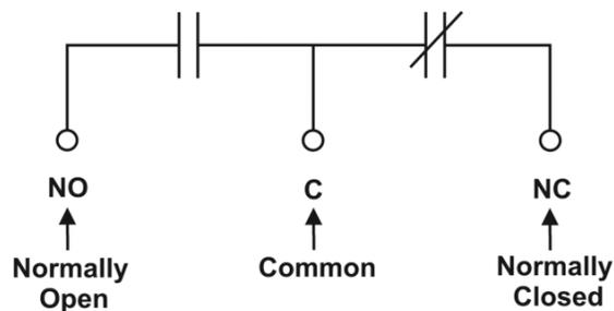
Relays can be programmed to energize or de-energize during an alarm condition (see controller software manual). When the controller reset button is pressed or power is lost, all relays de-energize.
