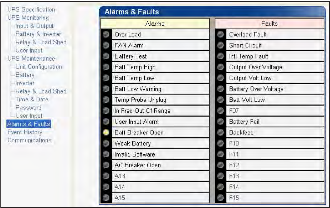
Figure 41 — Alpha UPS Monitor: UPS Alarms & Faults screen
