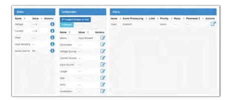
4. In the **Alarms** table, click the more details icon of the **Breaker/Fuse Open** alarm and configure as required.
