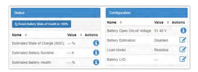
A battery run time prediction is performed while the battery is supplying power to the load. The controller collects data to estimate the time it will take the battery to be drained. If the battery estimation is enabled and the battery is sourcing current to the load, the estimated battery runtime if **AC Mains** is lost displays.
