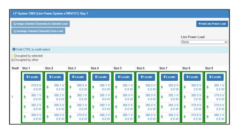
2. Select a load from the drop-down menu. The channels assigned to this load will be highlighted.
