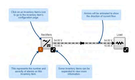
Figure 16-4 Interacting with the Power Flow
