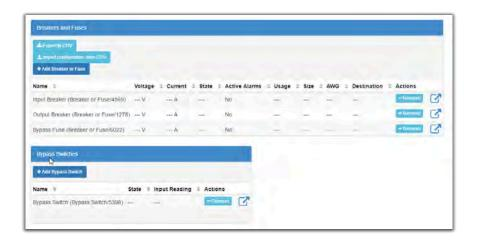
3. In the **Bypass Switch** table, set the **Name**, **Description** and **Input Source** values. When the value of digital input source is **Active**, bypass is in the **Bypass** state. When it is Inactive, the bypass is in the **Inverter** state. Alternatively, click the **Configure Bypass Switch** wizard to be prompted for the essential configuration required for the bypass switch to function.
