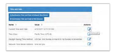
5. If setting the time and date using SNTP, first enter a valid SNTP server address, and then click **Synchronize Time and Date to Network Time Server**. If you do not want to use the SNTP server, clear the **Network Time Server Address** field.
