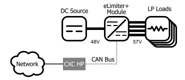
Note: Due to the remote location of down converter modules, they are not monitored by the CXC HP controller.
