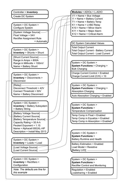
Figure 5-6 Quick Reference for Configuring a DC System
