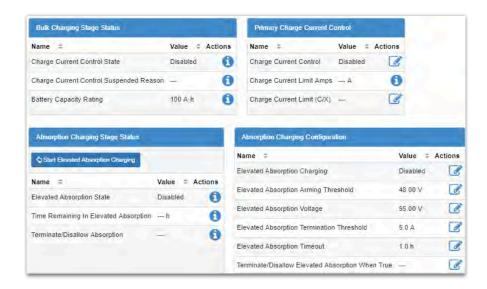
Lead acid batteries should be charged in three stages, which are constant-current charge, absorption charge and float charge. The constant-current charge applies the bulk of the charge and takes up roughly half of the required charge time; the absorption charge, also known as topping charge, continues at a lower charge current and provides saturation, and then goes into float mode.
