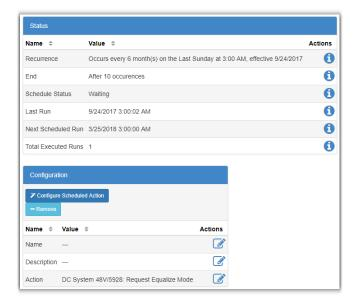
A **Scheduled Action** can also be triggered manually by clicking **Trigger Action Manually**. This is intended to be used for testing during configuration.
