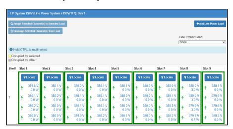
2. Using the **Line Power Load** drop-down list, select a load. A table displays detailed information about the load. You can modify the name, description, and other information about the load as well as do all load management tasks from this page.
