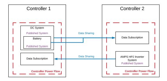
Components drawn on Power Flow that are managed by a different controller will have a reference to the **Data Subscription** they originate from. Clicking on these references will navigate to the user interface of the managing controller.
