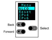
Figure 4-38 In-Shelf Controller Buttons: Horizontal Mount
