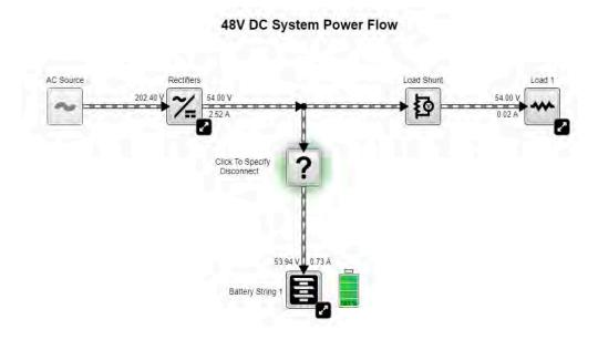
This feature can be disabled under Controller > Configure Controller > User Interface Preferences > Power Flow Configuration Suggestions.
