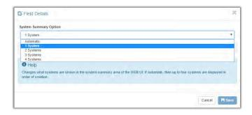
4. To change which system displays in the left most area of the system status bar, click edit for 1st system, and then select an option from the drop-down menu.
