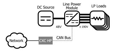
Figure 8-2 Example eLImiter+ System
