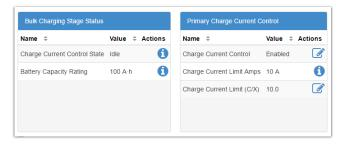
3. Set the **Charge Current (C/X)** limit to an appropriate value (for example,10-hrs). See your battery manufacturers' data sheet for charging recommendations.
