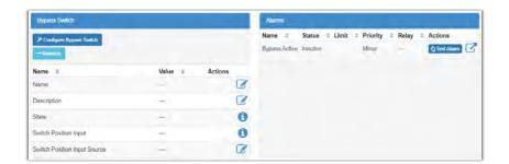
4. In the **Alarms** table, click the more details icon of the **Bypass Active** alarm and configure as required.
