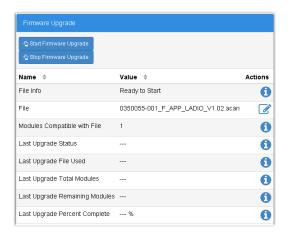
If an upgrade has been completed since the last restart, the bottom rows of the table will still contain information about that last upgrade until the **Start Firmware Upgrade** button is pressed.
