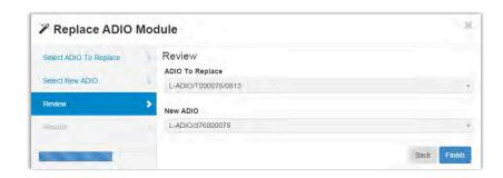
4. Click the **Finish** button to accept the change. The resulting table should have the new ADIO in it along with all of the mappings and configuration from the old ADIO.
