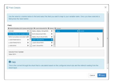
Once a field is clicked, the bottom area of the screen displays the name, value and additional information within the **Help** text.
