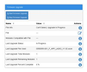
The firmware upgrade can be stopped if necessary. If you press **Stop Firmware Upgrade** button the controller finishes upgrading the current module so as not to leave it in a non-functional state. If multiple modules are queued, the next module will not be upgraded.
