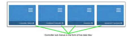
**Controller Status**: Provides the ability to reset the controller and view critical controller related information.
