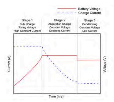
Figure 5-2 Three-Stage Charging Cycle
