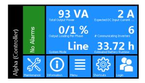
To access the wide data layout, go to **Controller > Shortcuts > Dashboard Config > LCD Dashboard Option > Wide Data Panel**. If there is more than one system on the controller. Switching to Wide Data Panel from "Automatic" is a two-step process. Once Wide Data Panel is chosen, a specific system must be selected so that the data values display for that specific system.
