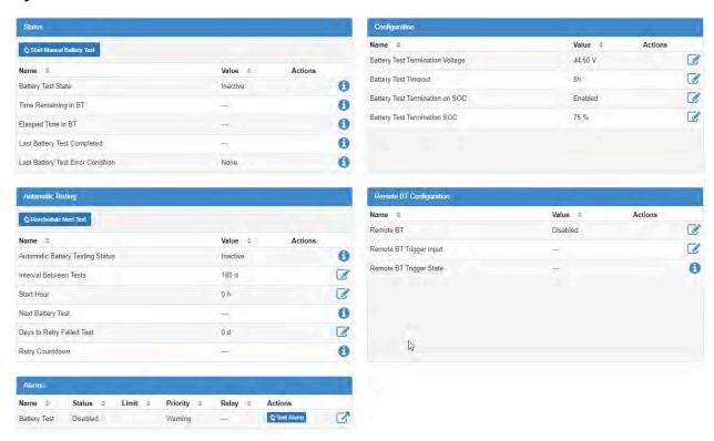
To run a manual battery test, the **DC System** must be in **Battery Conditioning** mode.
