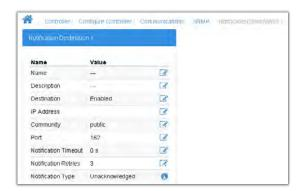
Clicking the edit icon on the IP address row allows you to insert an IP address of the monitoring destination.
