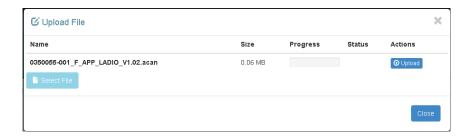
Once the file is uploaded, the dialog closes. The uploaded file is now visible in the **Firmware Files** table and available to upgrade a module.
