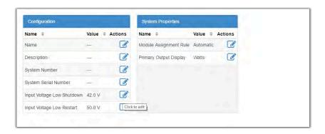
3. In the same table, set the Input Voltage Low Restart threshold to the desired value.
