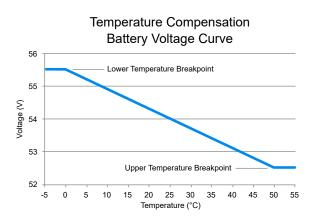
Figure 5-3 Temperature Compensation Voltage Graph
