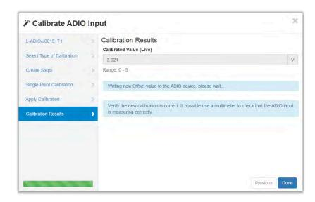
9. Verify that the new **Calibrated Value** matches the digital voltmeter reading. Click **Done** to close the Wizard.
