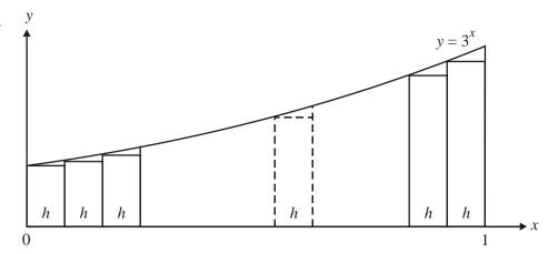
The diagram shows the curve with equation  $y = 3^x$  for  $0 \le x \le 1$ . The area A under the curve between these limits is divided into n strips, each of width h where nh = 1.
