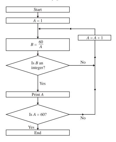
Implement the algorithm given by the flow chart above and state what the algorithm actually produces.
