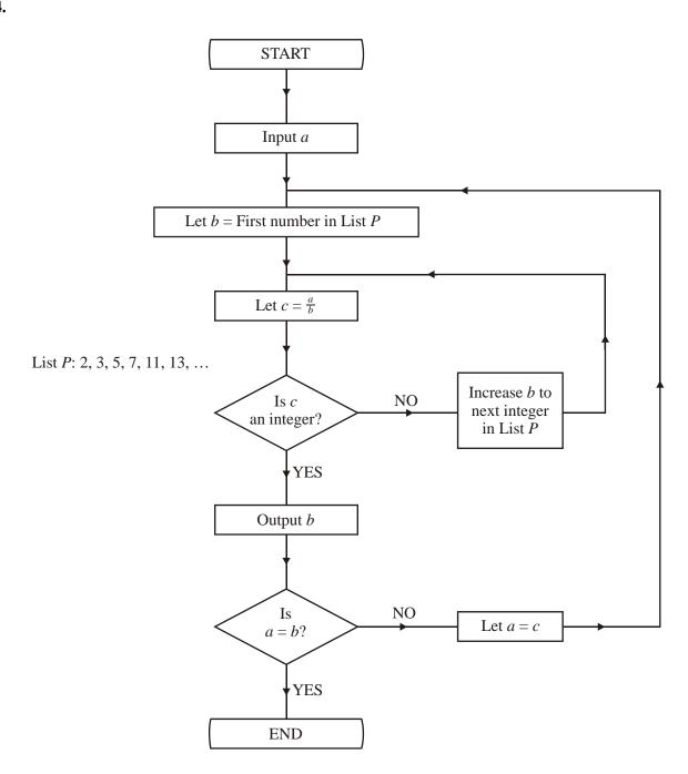
The diagram above describes an algorithm in the form of a flow chart, where a is a positive integer.
