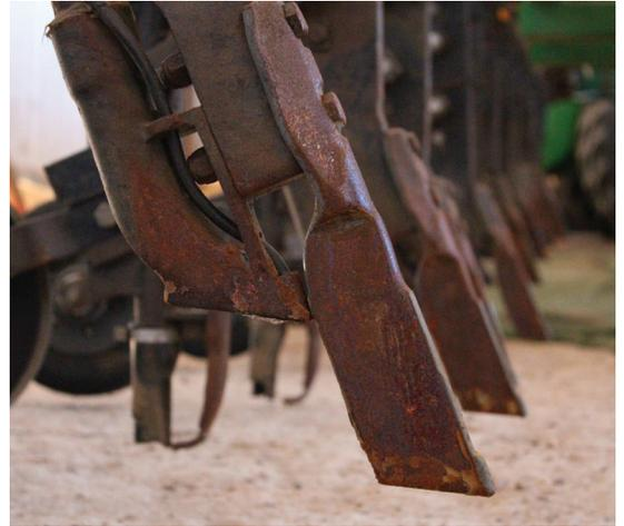
Figure 6: Sowing boot with liquid injection tube fitted.
