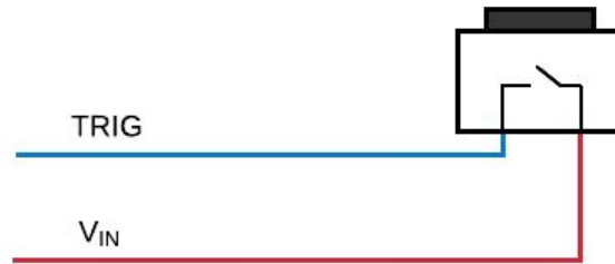
Figure 8 - External Button Wiring
